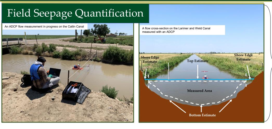
Conducting water balance on irrigation canals and using Acoustic Doppler Current Profiler (ADCP) devices for flow monitoring
