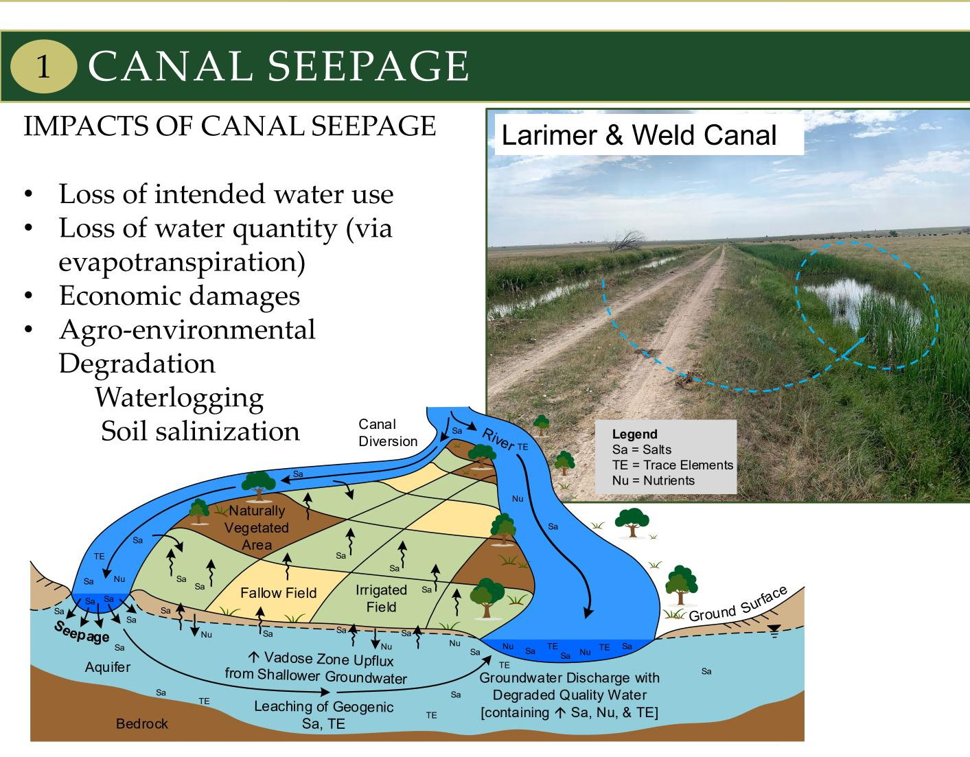
A conceptual schematic of water loss and negative environmental impacts from canal seepage
